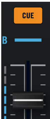
The CUE button on channel B
