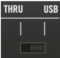
The THRU to USB switch.
