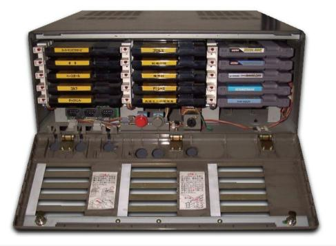
Strangely, the FamicomBox supports standard NES (not Famicom) controllers and Zapper light gun
